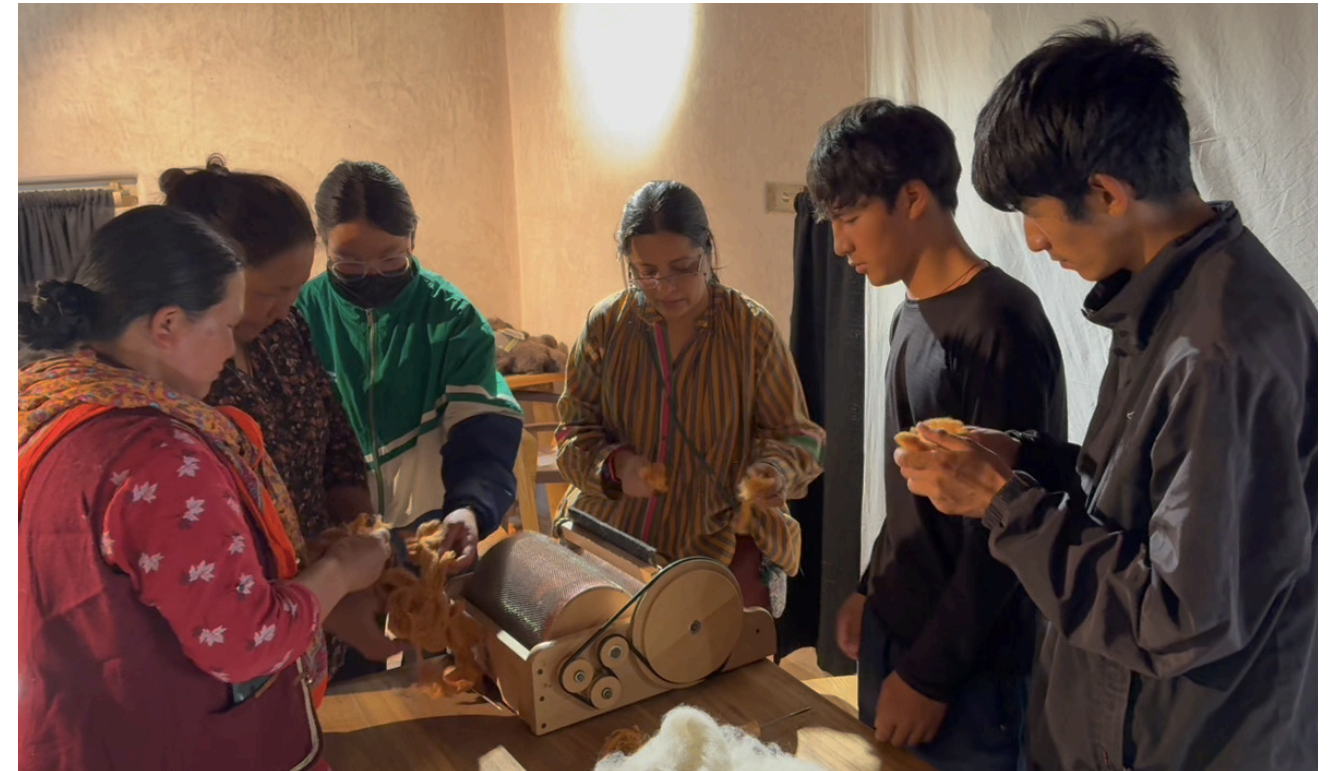
(Image on the left page): A functioning carding machine in Choglamsar, possibly the only one currently publicly accessible for use. It can card upto 5kg of wool per hour.
