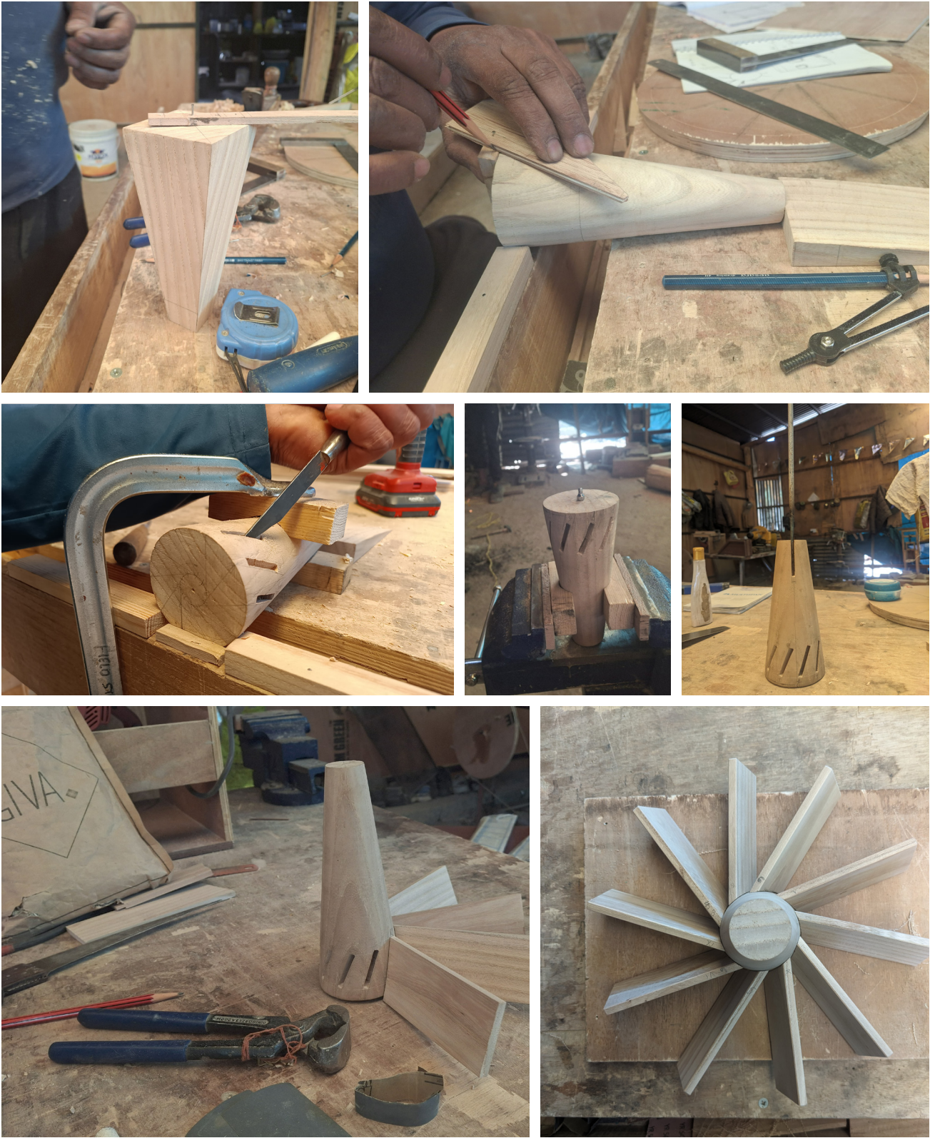
First row: Recreating the turbine (skuru) replicating the salvaged turbine from the site.
