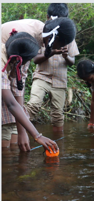
At Oothu, KMTR, these Roversians are measuring the stream's rate of flow using a floating ball.
